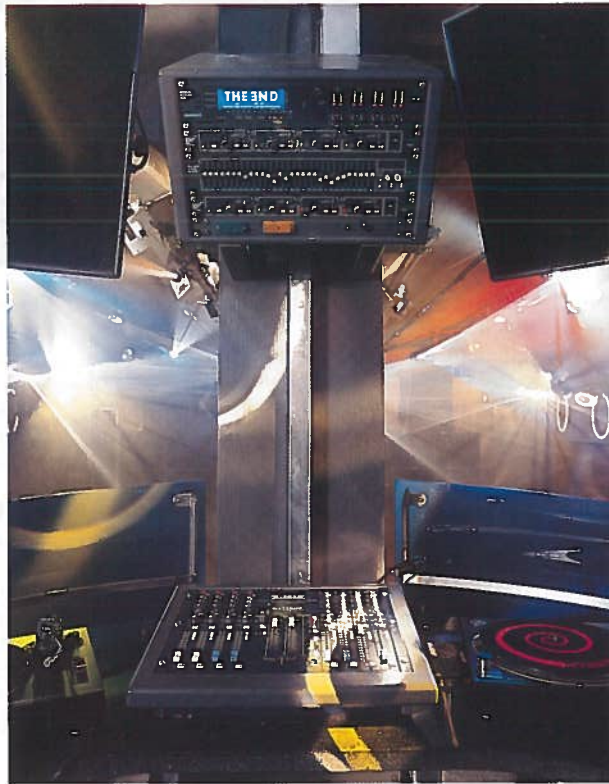
The Soundcraft D-Mix 1000 with the BSS Omnidrive and graphic EQs looming overhead.
